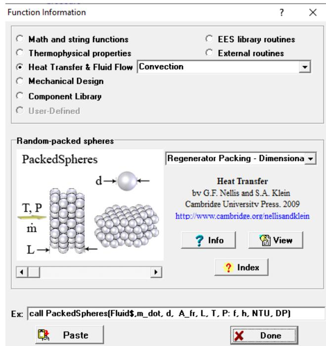
The properties required are computed using EES' internal property database and the heat transfer coefficient is computed using the PackedSpheres procedure.
