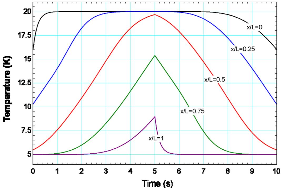
If the Automatic Update feature is selected in the plot then it is possible to change an input in EES and simply re-run the Macro to see how the temperature distribution changes. For example, if the mass flow rate is doubled, the new temperature distribution is shown below.
